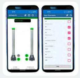
Detection and signaling parameters can be easily set via the OPENGATE App designed for smartphones or tablets based on Andriod or iOS operation systems.
